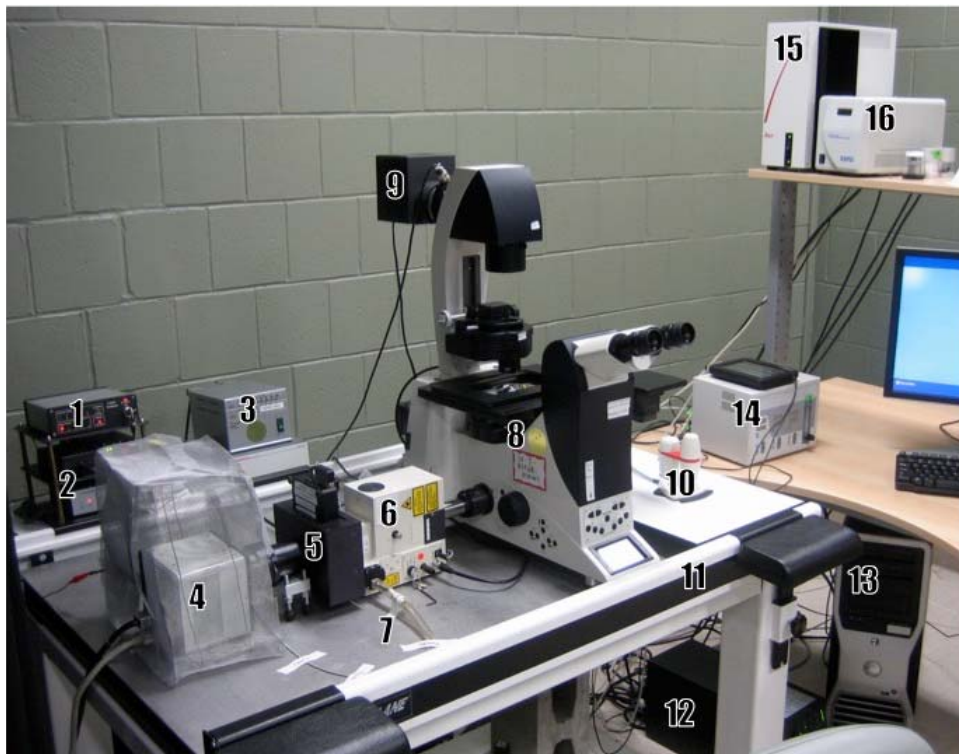
Fig 1: Basic components of the SD2 microscope; brand names in italics.
